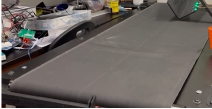
Figure 31. The treadmill used to transport waste into the system.
