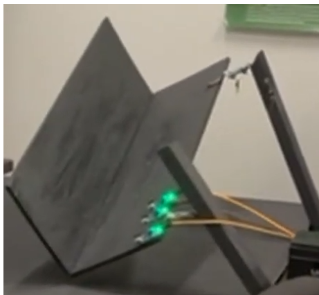
Figure 32. Sensor placement on delivery chute.
